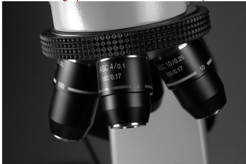
Figure C-4. A typical microscope nosepiece with objective lenses
