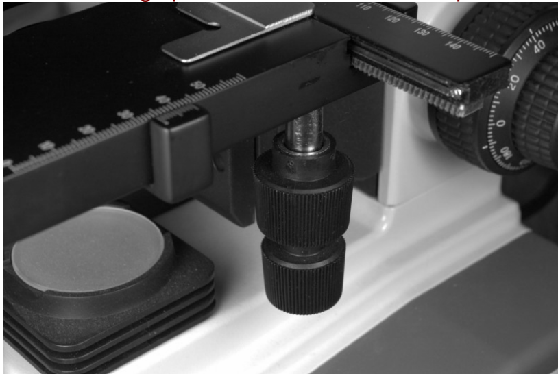
Figure C-7. Knobs control the X- and Y-axis movements of the mechanical stage
