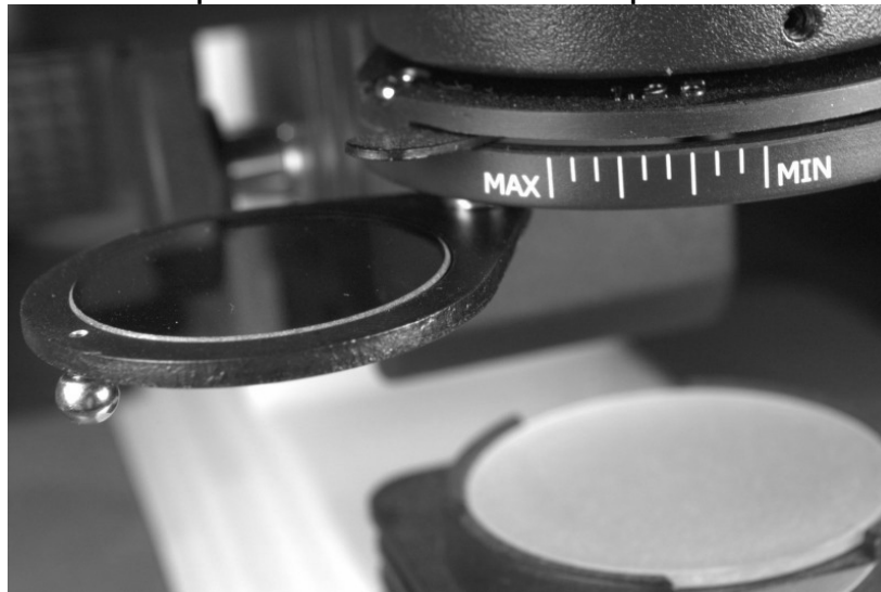
Figure C-8. The diaphragm control lever (note the swing-out filter holder to the lower left)
